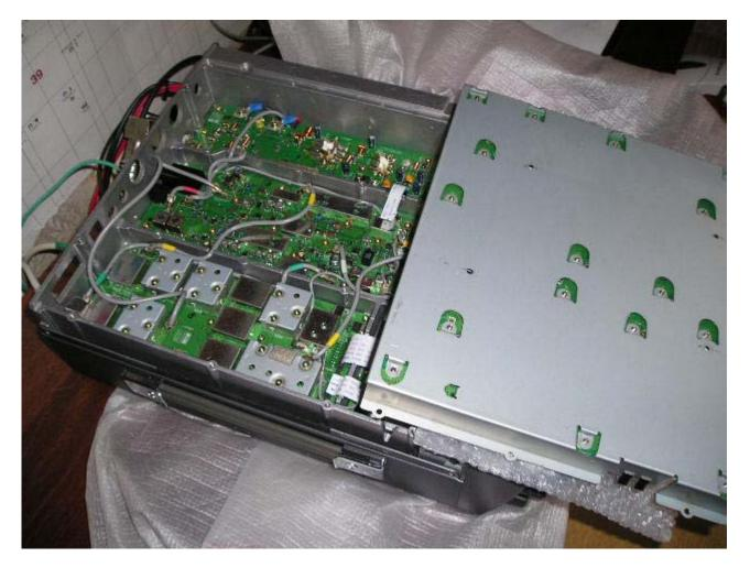
*We further unscrew 13 screws "of [samorezov]" of fastening the module "VU RF", see. the photo:*
