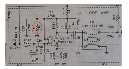
I think commentary they are superfluous, by the way in the European version everything is made correctly! Well and now recommendation - as to reach the resistor Of r15, which must be replaced by the analogous SMD resistor with a resistance of 22-36k. The dismantling of transceiver - you will unscrew 10 screws of fastening lower protective housing, and remove it:
