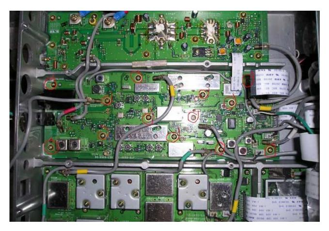
And having accurately disconnected connecting joints we extract module, see. the
