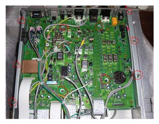
After unscrewing 10 screws "of [samorezov]" of fastening the block **TX-RX UNIT** we accurately raise it even we turn over, you look the following photo:
